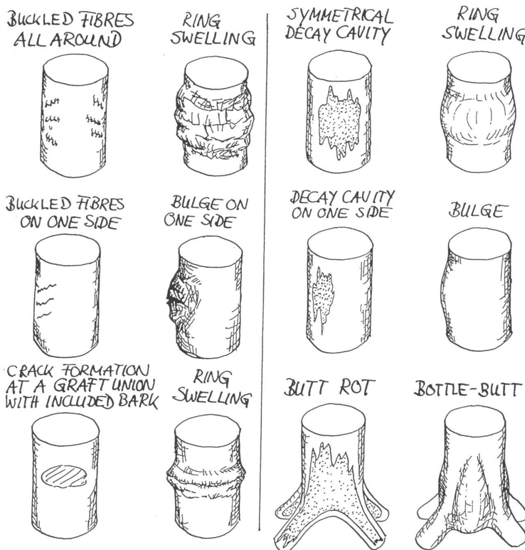
Fig 105. Examples of swelling and bulge formation in response to various internal defects.
