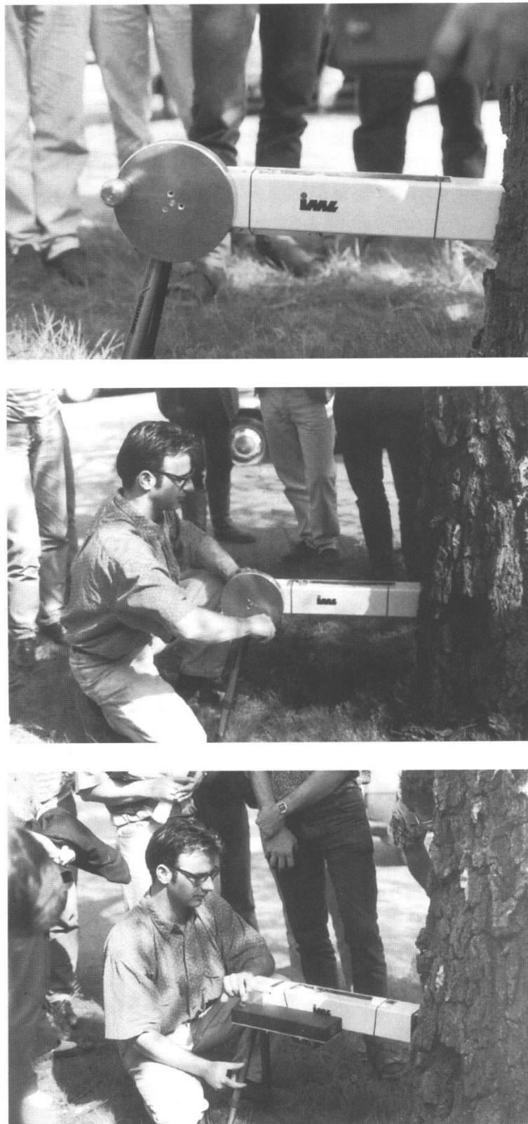
Fig 129. The 'Resistograph' M is the purely mechanical version of the tried and tested 'Resistograph'. It can be driven either by hand by means of a crank or by an electric motor. The needle drill is 30 cm long. The inner workings of the drill are entirely mechanical with no electronics (Demonstrated by Bernd Lüll).
